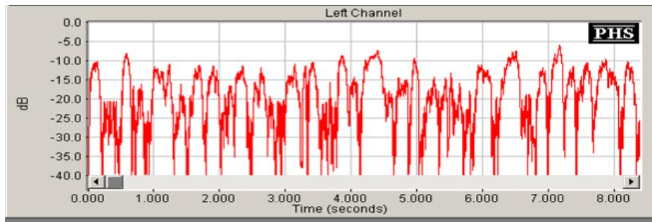
**Figure 3: Pulse pattern from an operational wind farm**
