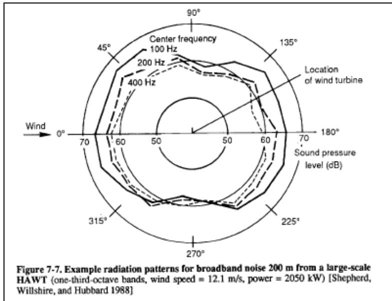
Figure 7-7. Example radiation patterns for broadband noise 200 m from a large-scale
