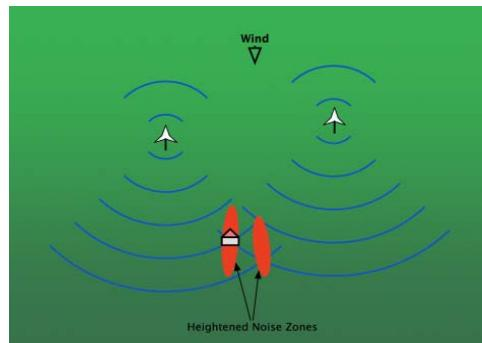
Figure 18: Noise from 2 turbines creating Heightened Noise Zones
