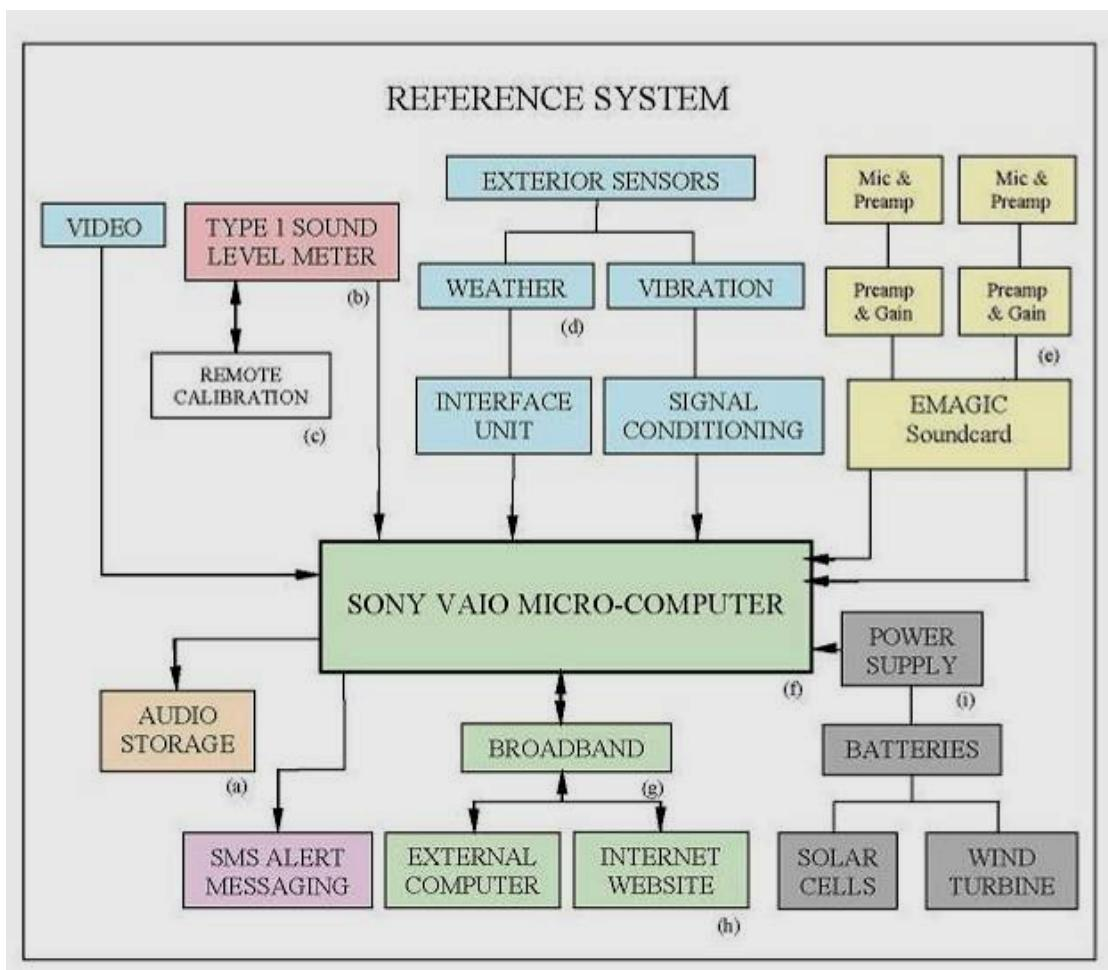
**Figure 1:** Reference sound recording system
